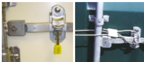
DHS may require shippers to use "high-security seals," such as bolts (left) or cables on inbound containers
